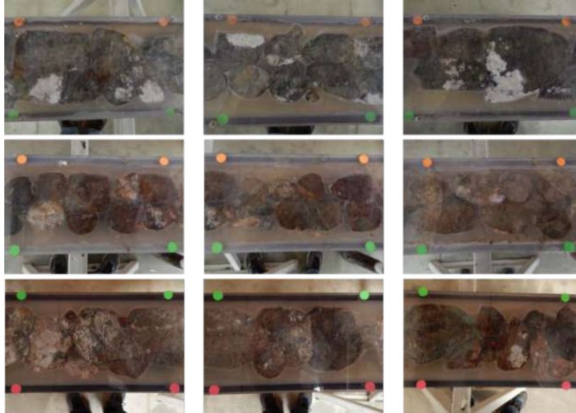
Typical occurrence and distribution of gypsum (white or light-colored minerals) in post leach photographs from core-box leach tests. Samples are from Martin, Upper Abrigo and Lower Abrigo formations. Dots of the same color are approximately 12 inches apart. Source: Excelsior
