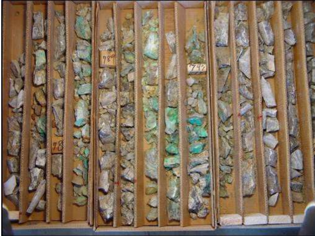
Figure 7-8: Photograph of Typical Oxide Mineralization for North Star Hole J-9: 780 to 806 feet
